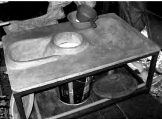
Figure 3: Locally made urination/defecation separation toilet (household scale) 13
