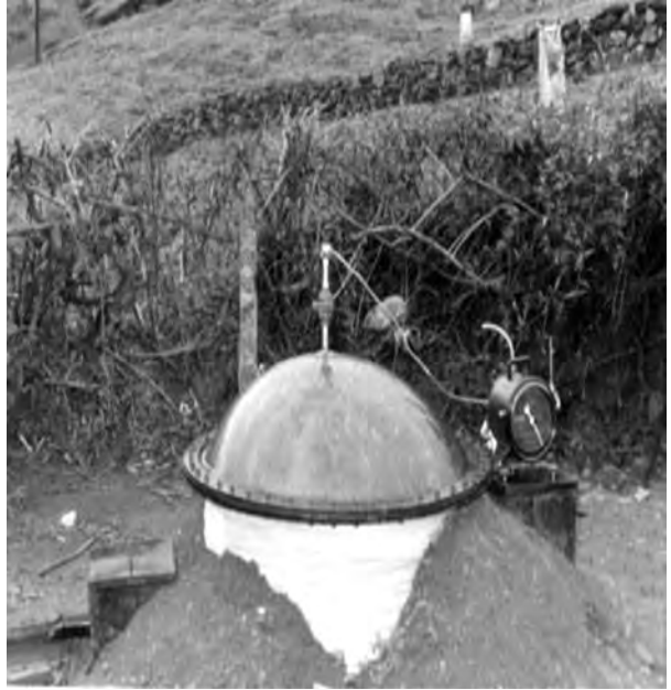
Figure 4: Localized (self-sufficient and contained) anaerobic methane digester 14
