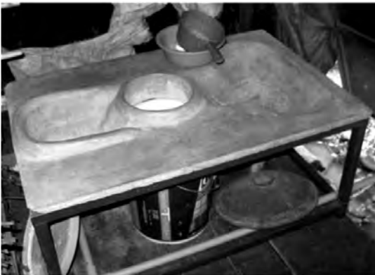
Figure 3: Locally made urination/defecation separation toilet (household scale) 13
